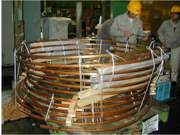
High-Pot. leak test
