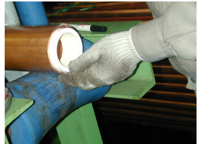
Insert MgO to copper tube
