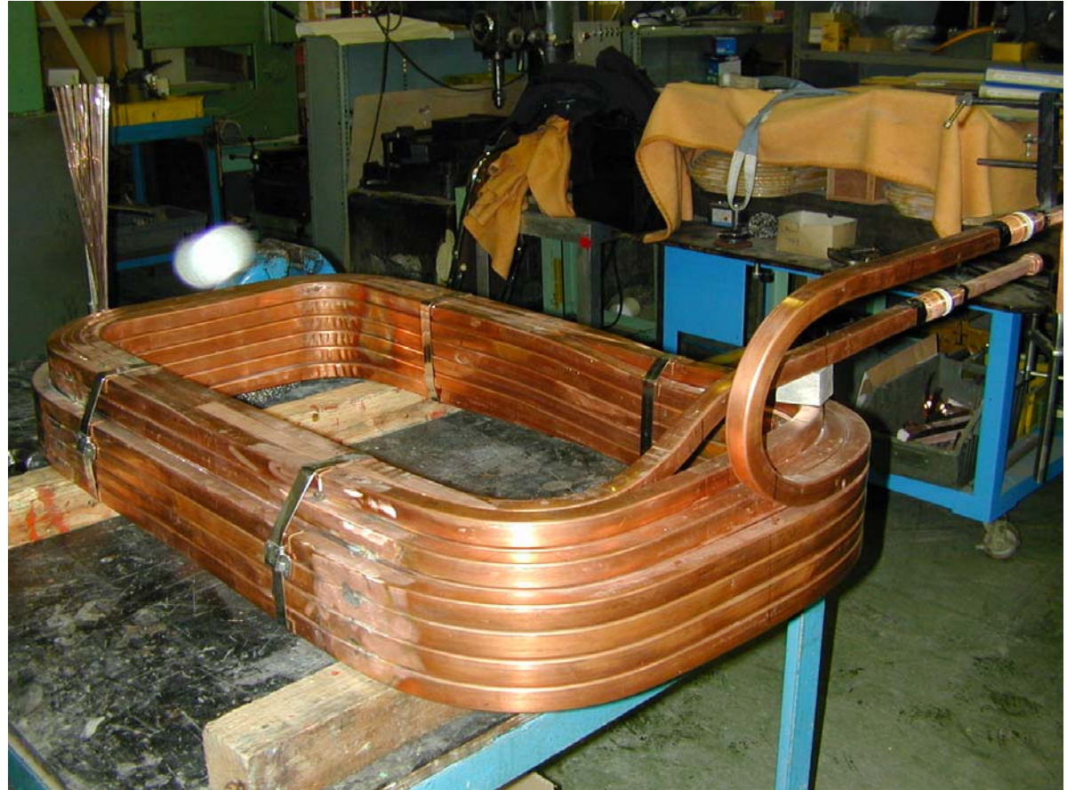
The first coil of 60m-2500A HC-MIC
