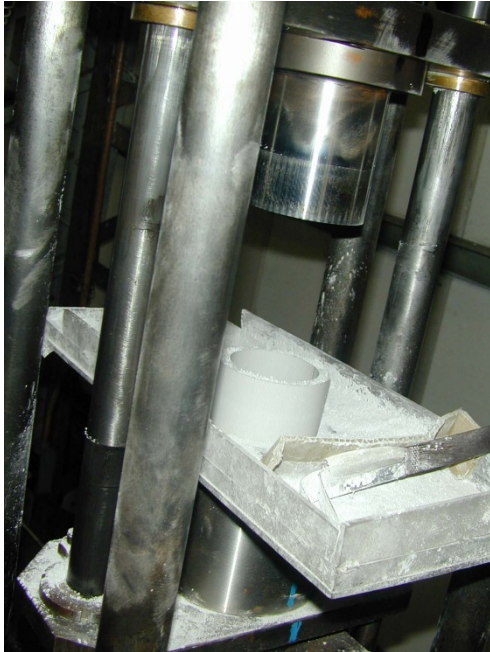
Hydraulic Press on MgO powder
