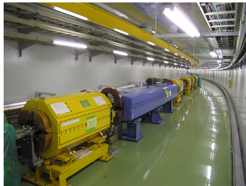
50 GeV Synchrotron. Special lattice structure to avoid transition energy.
